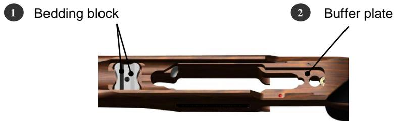
Gently insert the barreled action into the stock, but do not insert the action screws **5** yet.
